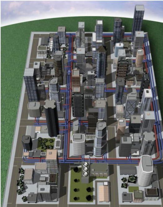
Figure 1 – District Energy Distribution System
